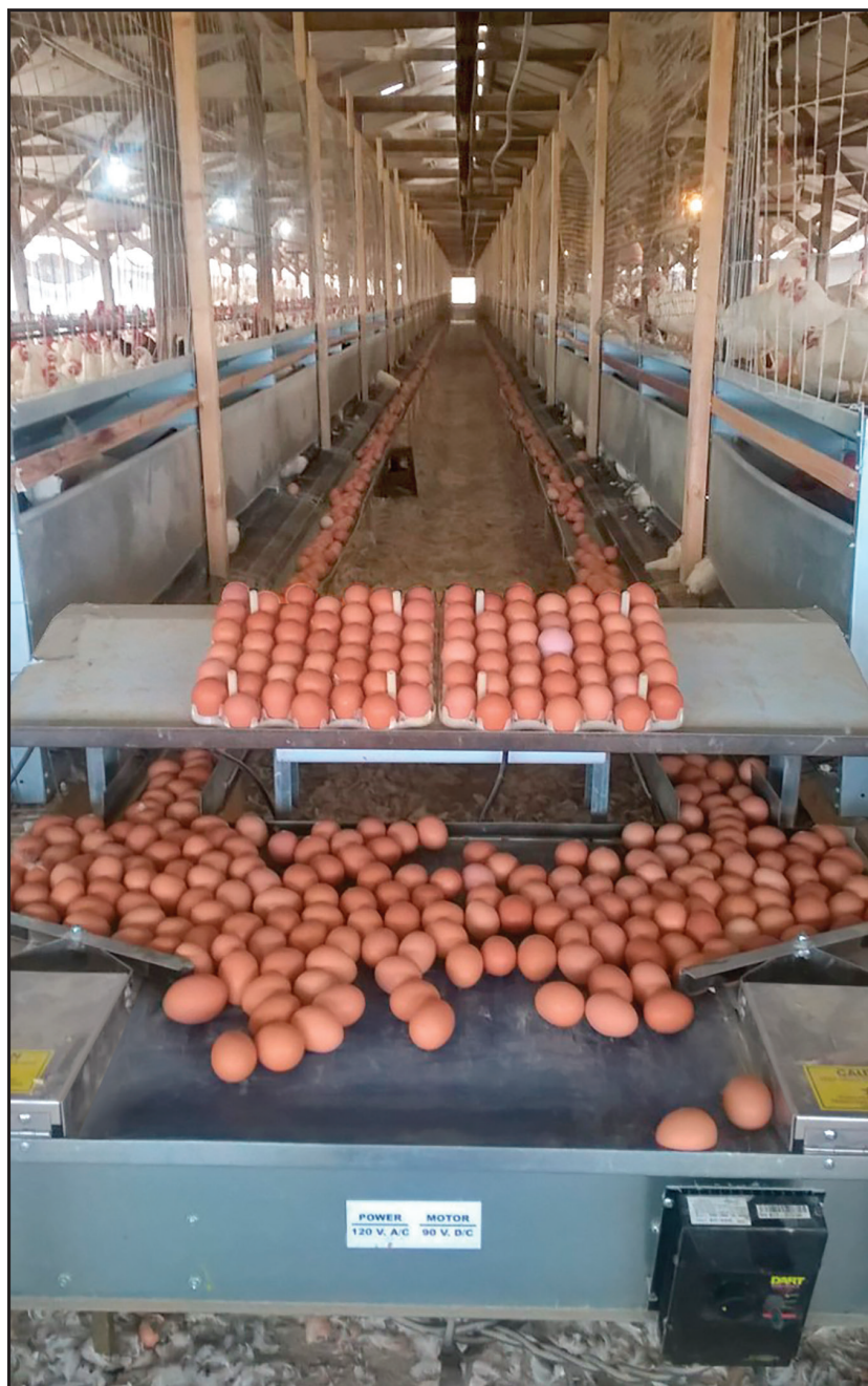
Variable speed belt drive. Hand gather option shown, but cross conveyor collector available.
